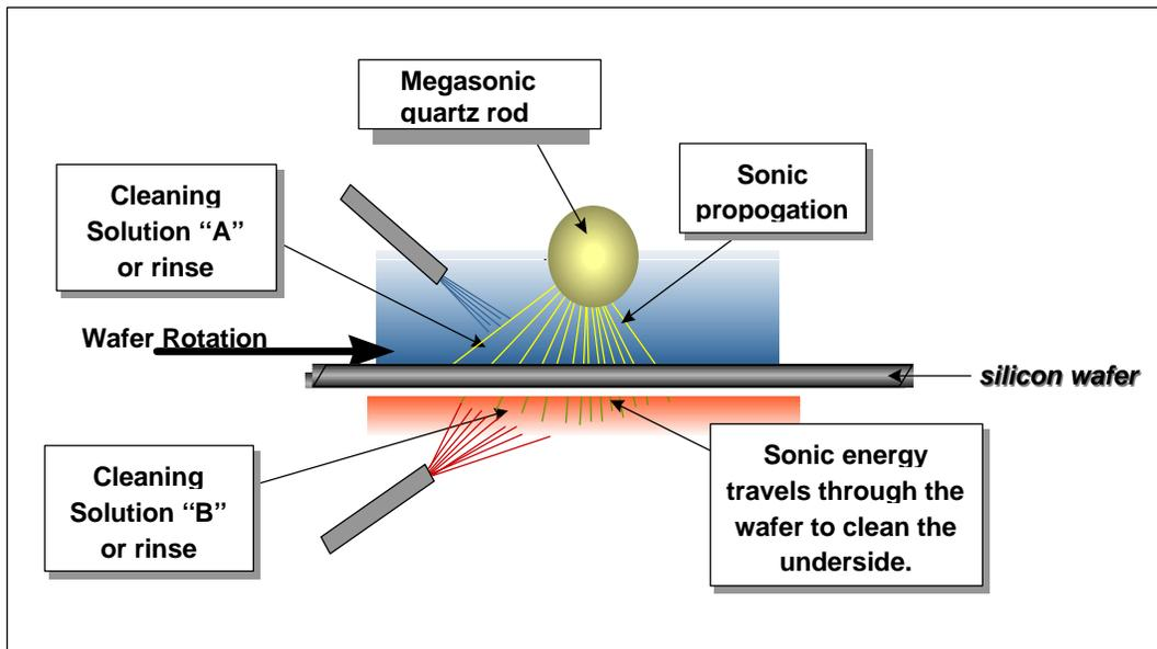
**Figure 2.** Schematic - megasonic energy propagation and liquid distribution.
