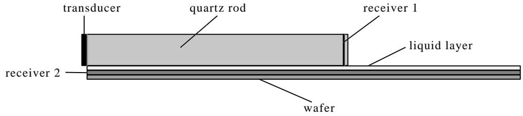
**Figure 5.** Schematic used for 2D simulation
