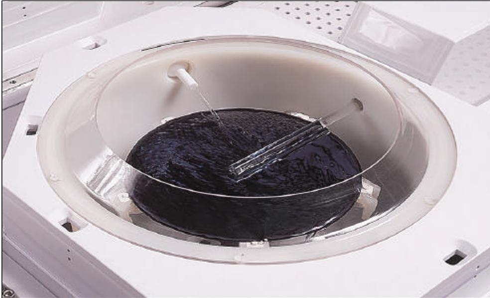
**Figure 1.** Cleaning module showing the quartz rod projecting over the wafer.
